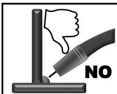
**Characteristics:** Small Convex weld possibly **with** bulging sides/cold lap and/or an inconsistent arc.
